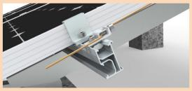
Step9: Install the grounding lug on each rail and run a grounding copper wire between each lug.
